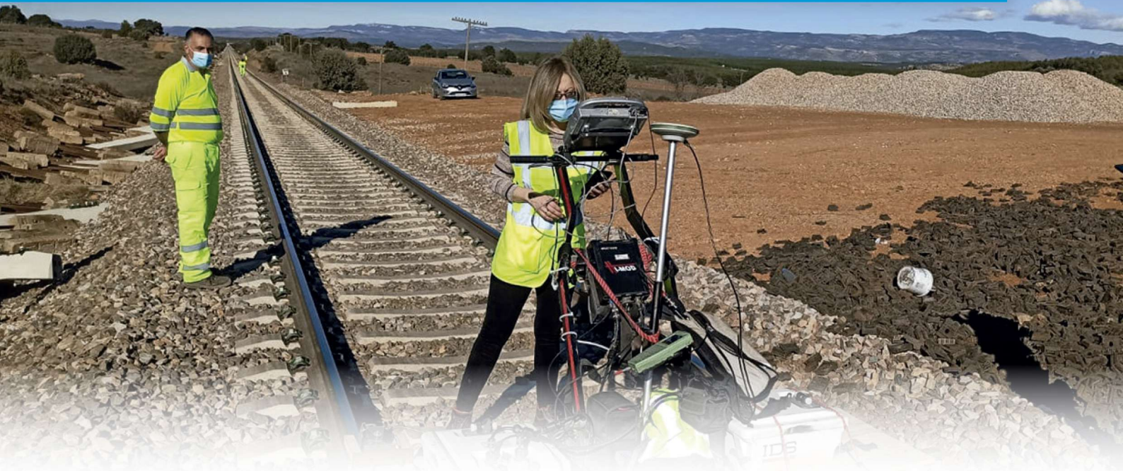
Real-time testing of a prototype of the track inspection vehicle designed
